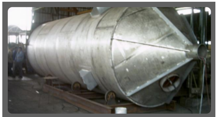
Fabrication / Installation of Degumming Tank
